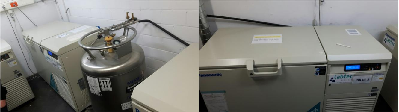
Freezers at -150 °C and a liquid nitrogen safety system in case of technical failure.
