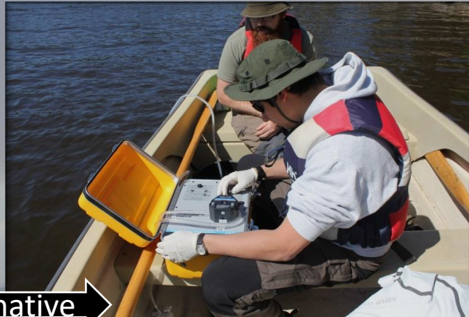
Battery driven easy portable water sampler (all in one box system, expensive)
